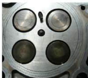
Direct injection cylinder head with fuel injector & heater plug
